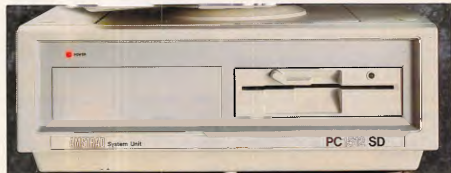
The standard unit contains a single floppy disk drive unit
